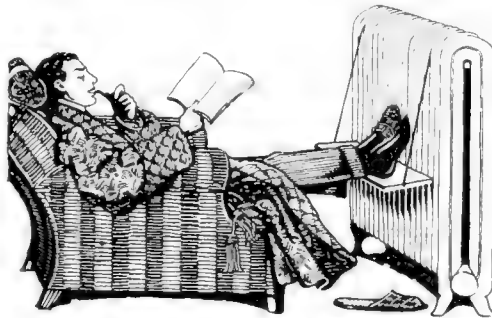
A shelf supported by long hooks attached to radiator connections for a foot-warmer
